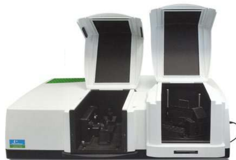
PerkinElmer LAMBDA 850+/1050+ with TAMS Accessory.
